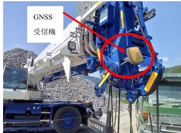
図-3 GNSS 受信機の取付け位置 (Installation position of GNSS receiver)
